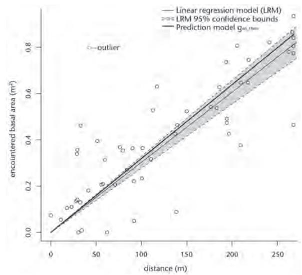
Fig 6 The cumulated real encountered basal area ( $g_{en\_real}$ ) from its starting to its stopping point versus the real planimetric distance travelled from the release point for each rock (depicted as black circles). The figure further presents the linear regression of  $g_{en\_real}$  with the 95% confidence bounds and the predicted basal area encountered by the falling rocks.
